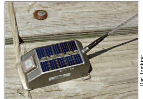
This solar powered transmitter will allow us to track the movements of a young eagle for up to several years before it falls off.
